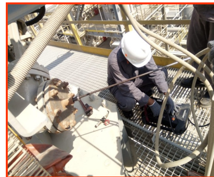
Stack Emission Testing
