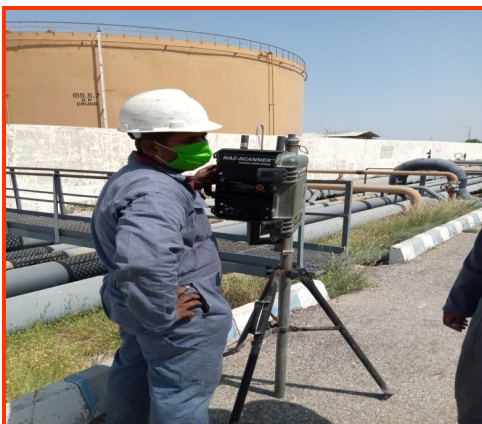
Fugitive Emission Testing
